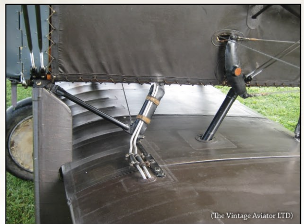
Port lower wing joint showing the tubes running out to the pitot head.
