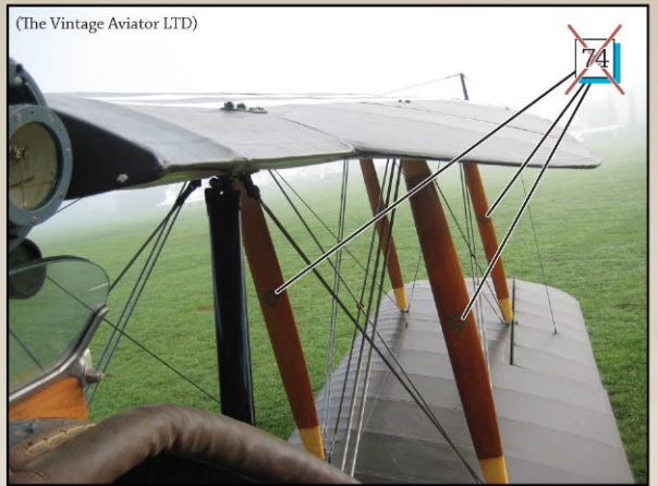
A pilot's eye view along the starboard wing showing strut decals and aileron control cable details.
