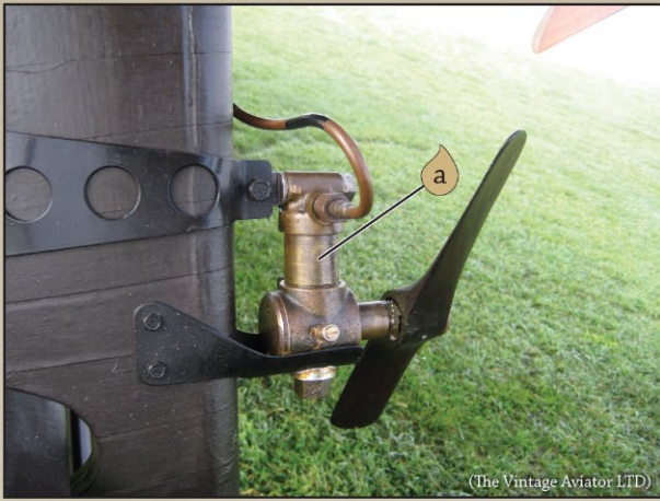
Wind driven air pump for providing pressure to the fuel system.
