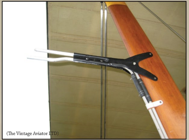
Pitot tube detail on port wing outer front strut.
