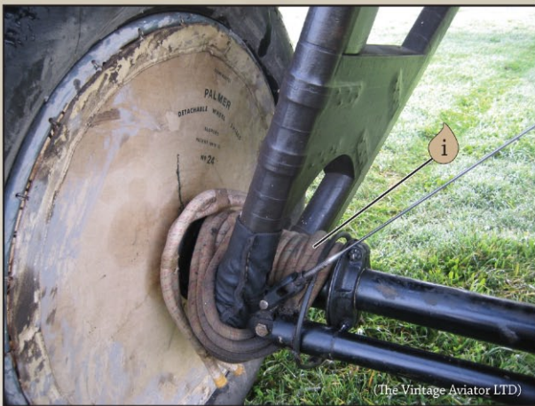
Right side wheel detail showing re-inforced undercarriage struts. Note the bungee shock cord and axle retaining wire.
