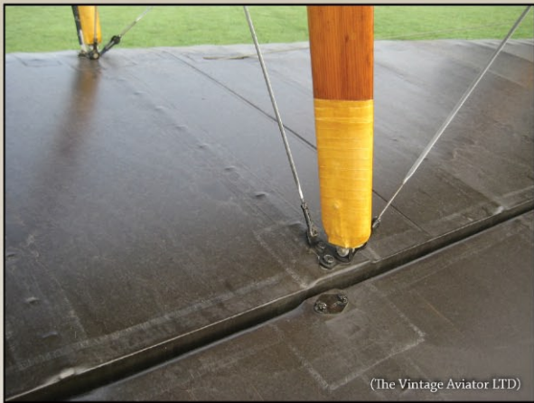
Port lower wing outer struts showing yellow reinforcing tape which should probably be Clear Doped Linen i .
