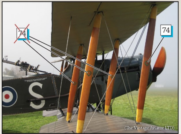
Starboard wings showing useful rigging details. See page 22 for a discussion on the over application of Bristol factory decals.
