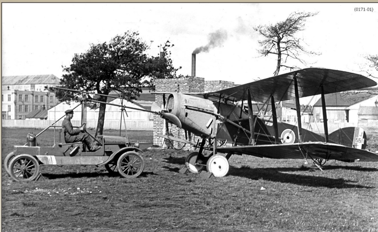
A Hucks starter truck is about to start Bristol F.2b Fighter Mk.II J6611. Note the Holt landing flare brackets and white(?) wheel cover. The Hucks starter truck was based on the ubiquitous Model T Ford and was widely used after the First World War.
