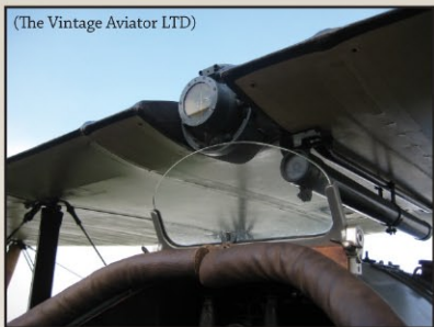
(The Vintage Aviator LTD) Windscreen, Aldis sight and Mark 5/17 compass details. Note the leather cockpit padding join at the centre.
