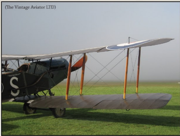
Starboard wings showing useful rigging details. See page 22 for a discussion on the over application of Bristol factory decals.
