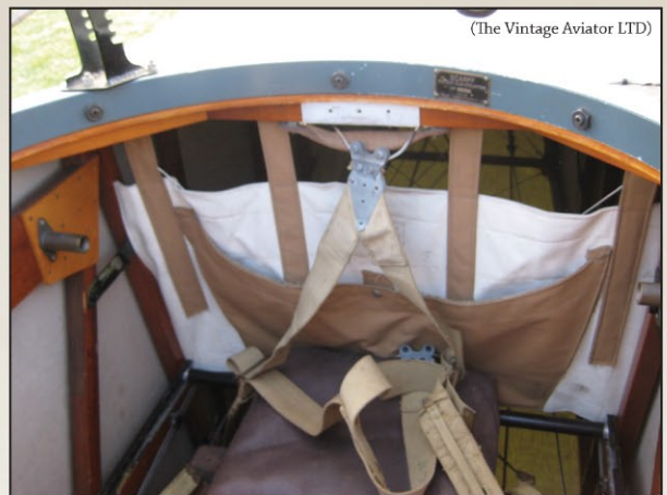
(The Vintage Aviator LTD) Rear of observer's cockpit showing the cloth screen and storage pockets, usually used for Lewis gun magazines. The 4 point safety harness shown here is not appropriate for our model.
