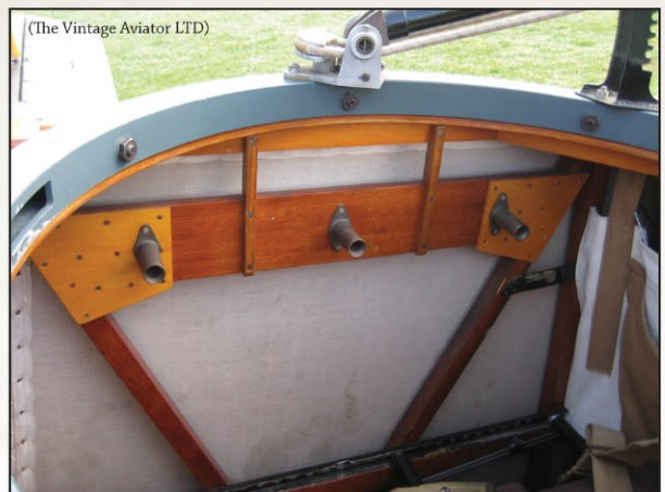
(The Vintage Aviator LTD) Right side of observer's cockpit showing mounts for spare Lewis gun magazines. Note the interior colour of the fuselage linen.
