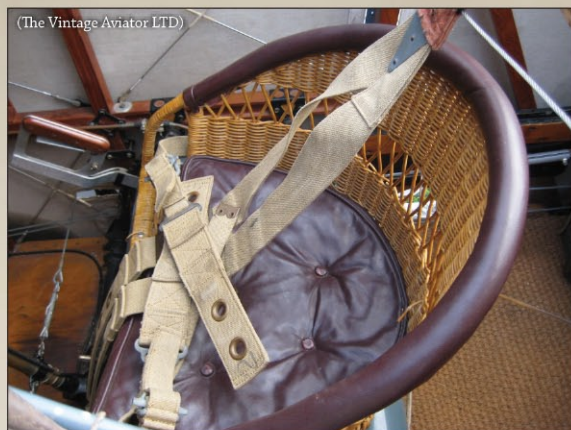
Pilot's wicker seat details, note the 'modern' 4 point Sutton safety harness not appropriate for our model.
