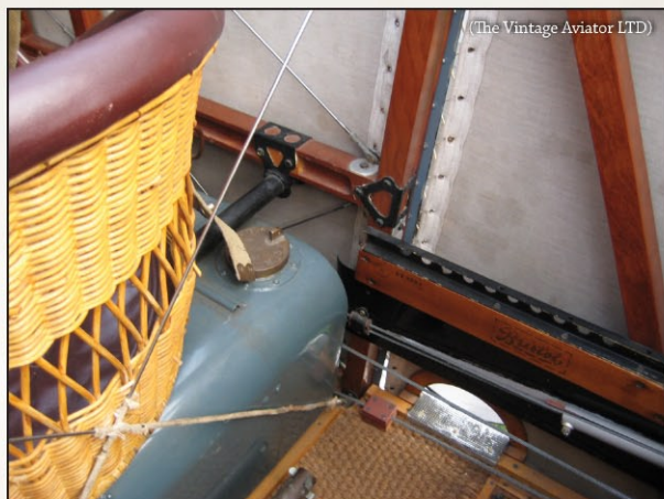
(The Vintage Aviator LTD) Rear of pilot's seat showing the rear fuel tank and fuselage foot step details.
