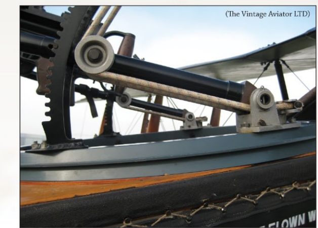
Scarff ring details, note the twin Lewis gun mounting.
