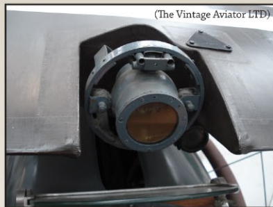
(The Vintage Aviator LTD) Mark 5/17 compass mounted in cut out at rear of upper cabane wing section.
