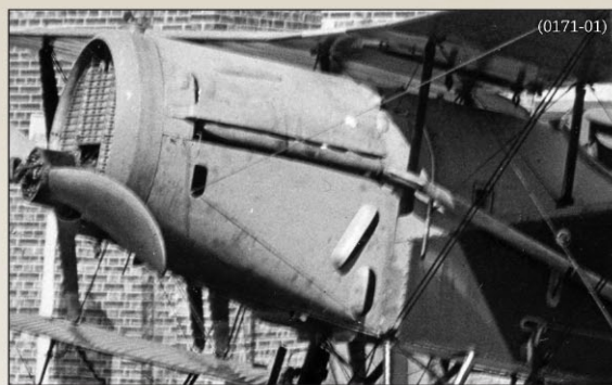
Engine cowling details from Bristol F.2b Fighter Mk.II J6611 as seen on pages 22 & 26. Note the slightly reduced size of the front cooling slot.
