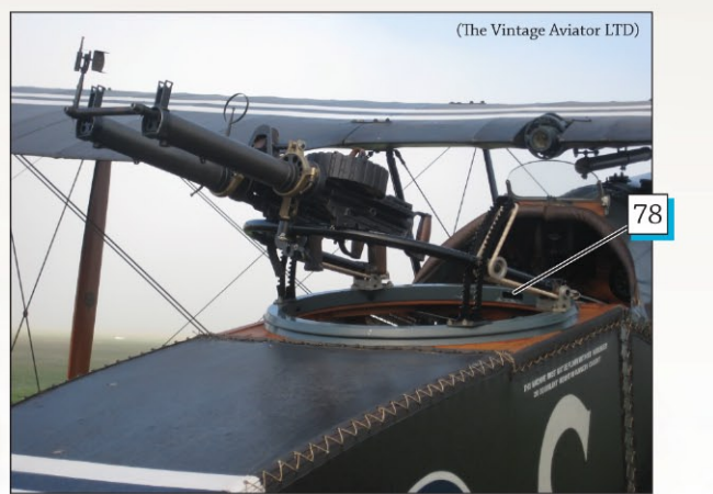
Scarff ring details, note the twin Lewis gun mounting.
