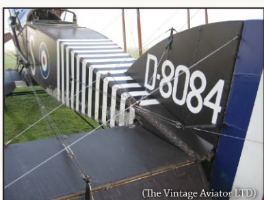
(The Vintage Aviator LTD) Tailplane showing the various control cables and RAF rigging wire details.
