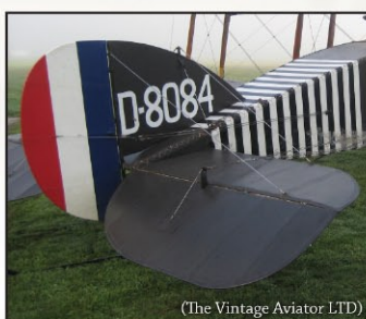
(The Vintage Aviator LTD) Tailplane showing the various control cables and RAF rigging wire details.
