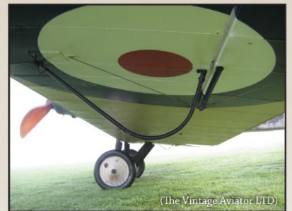
(The Vintage Aviator LTD) Wing skid detail.
