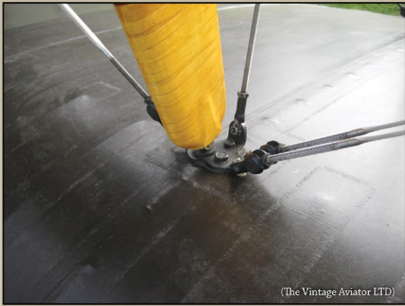
Port lower wing inner front strut showing rigging wire detail.
